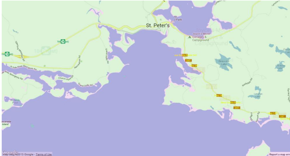
Figure 6. Map showing projected 2 meter sea level rise, created in quantum GIS software. Areas in pink represent inundated areas.
