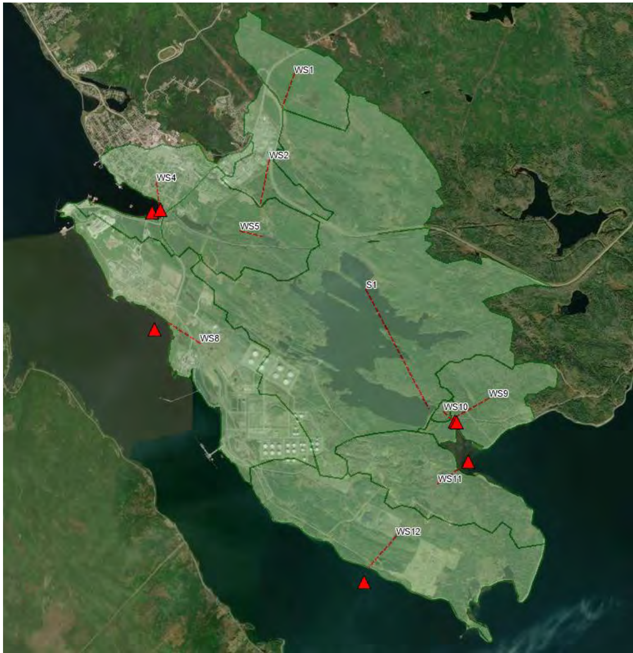
Figure 3-24: Hydrological model layout for study area watersheds. Red triangles indicate locations where flow time series are generated to serve as inputs for the coastal model (see Section 3.6.4).
