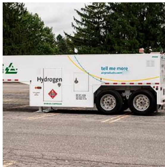
Figure 9: Portable hydrogen refueling station
