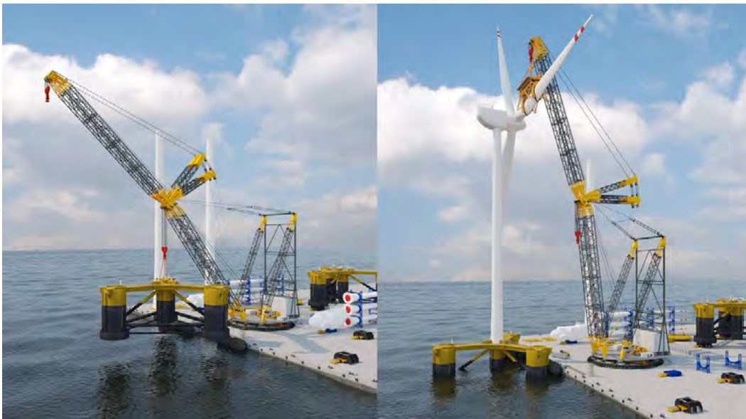
FIGURE 10: RING CRANE, SOURCE: MARINE LINK
